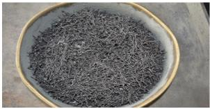
Fig -1 Steel fibres
