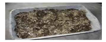
Fig -3 Basalt fibres
